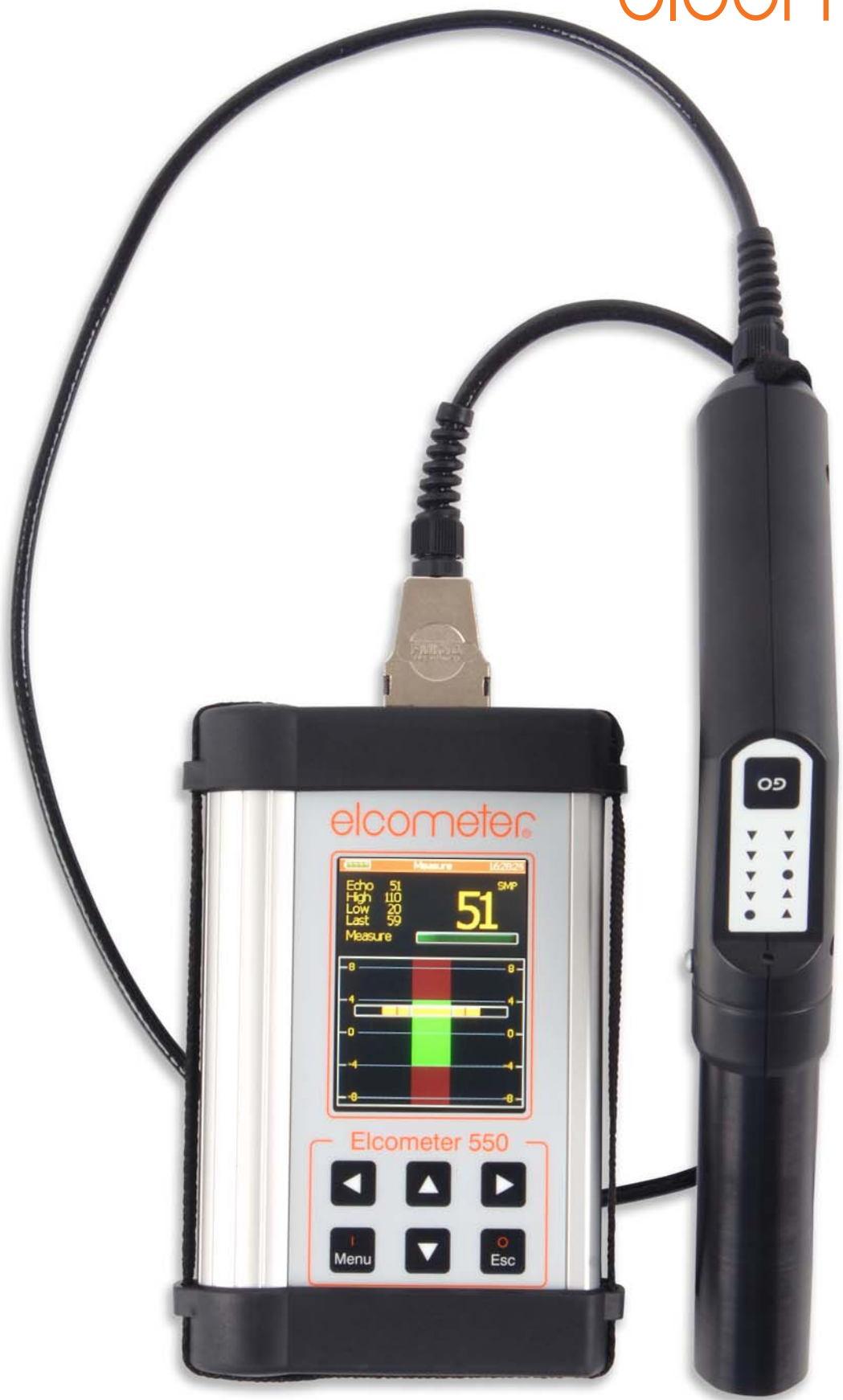
Elcometer 550 Non-Contact Powder Thickness Gauge
