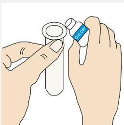
1. Remove cap from CHLOR\*EXTRACT solution bottle and pour entire contents into the test sleeve.
