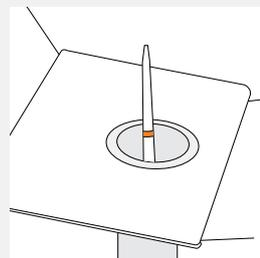
4. Insert sleeve with extract solution and titration tube into the hole previously made in the box lid and wait 1½ minutes.
