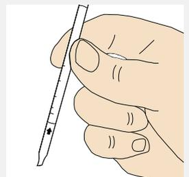
5. Immediately remove and read the number on the titration tube at the interface of the colour change. Pink is normal, white is the chloride level.
