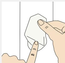
2. Firmly apply test sleeve to test surface, allowing extract solution to come into contact with test surface.
