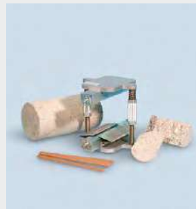
SPLITTING TENSILE CONCRETE CYLINDERS
