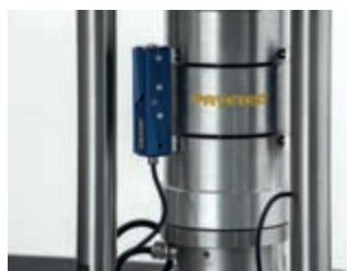
B203 verification device with on-specimen LVDTs and load cell
