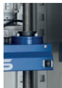
B220-12 20 kN Load frame with motorized crosshead
