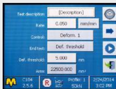
C104-10N Set up of customized compression test
