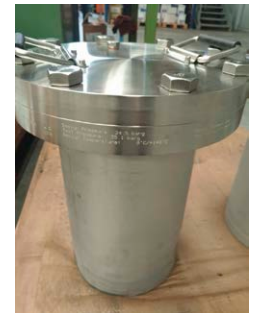
Pressure vessel is CE and ASME certified to resist at a design pressure of 24.5 bar at 148 °C
