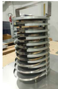
Sample rack for testing up to 10 samples at the same time, in a flat position.
